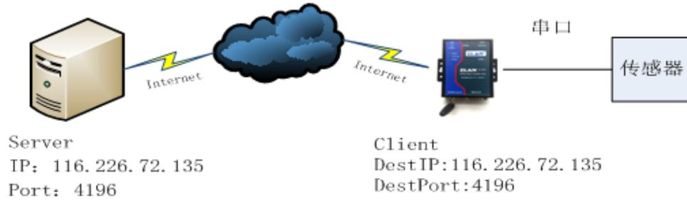
FIG. 21 Networking Structure Diagram
