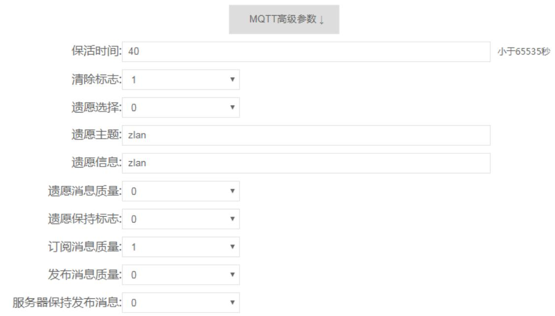
The screenshot shows a configuration interface for MQTT advanced parameters. At the top, there is a button labeled "MQTT高级参数 ↓". Below it, several parameters are listed with their current values and input fields:
